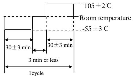
Performance: The capacitors shall meet the following specification after 5 cycles.
